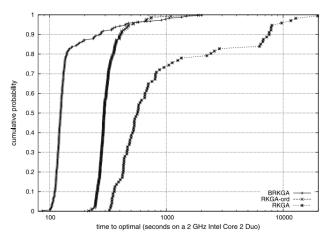
Time to target plots compare running times needed to find the optimal solution of a 220 element covering by pairs problem with a BRKGA and two variants of a RKGA
