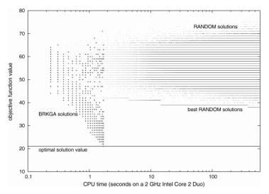
Comparing a BRKGA with a random multistart heuristic on an instance of a covering by pairs problem
